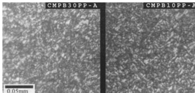
**Figure 7** Comparison of the spherulitic core morphologies in CMPB10PP-A and CMPB30PP-A.
