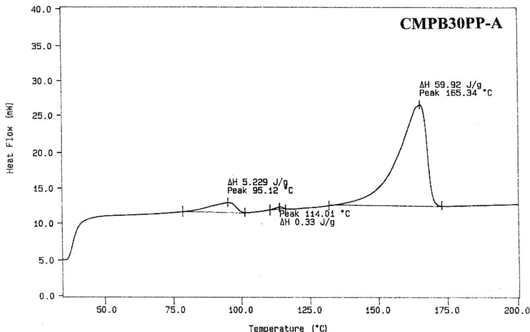
Figure 11 DSC thermogram of CMPB30PP-A.
