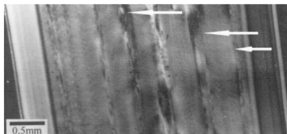
**Figure 6** Whole longitudinal cross section of SCPB30PP-A. The white arrows point to interfacial features.
