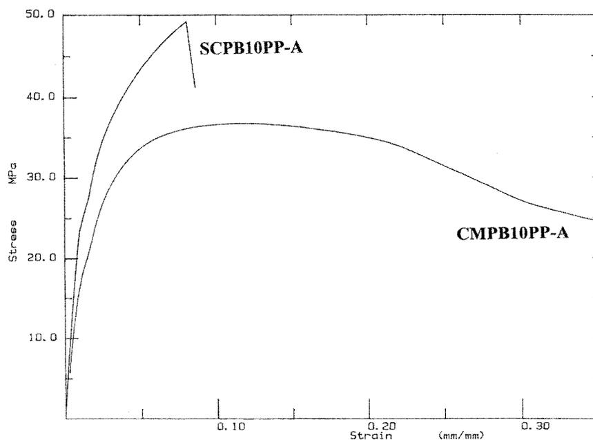
**Figure 1** Stress-strain curves for CMPB10PP-A and SCPB10PP-A.
