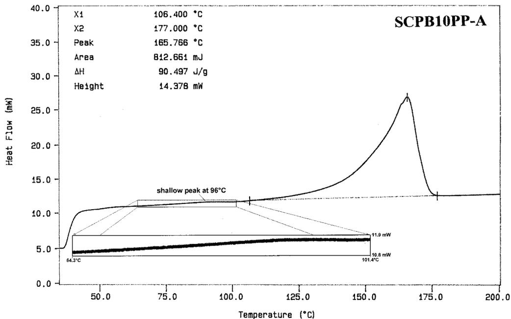
Figure 10 DSC thermogram of SCPB10PP-A.
