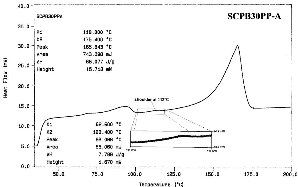
Figure 12 DSC thermogram of SCPB30PP-A.
